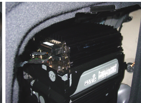
Picture of amplifier in -2006 Model. A different cable set is required.
