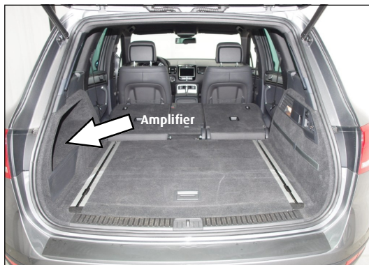
Picture of amplifier location
