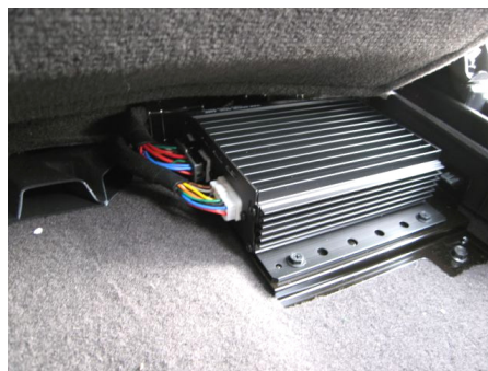
Amplifier location in Santa Fe
