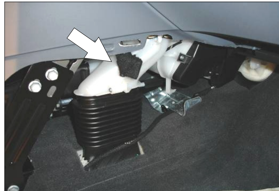
The picture show the location of the VDA connector in a Saab 9.3 Sport.
